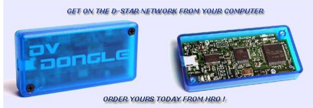
The DV Dongle costs about \$299. It is essentially an AMBE chip plugged on a card that allows a user to connect to any DPlus enabled gateway. In short if the repeater has a gateway with DPlus on it, you can connect to it.
